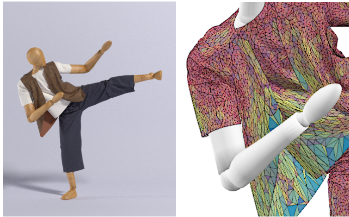
Figure 3.7: The anisotropic remeshing algorithm of Narain et al. [NSO12] allows detailed wrinkles in cloth to be resolved accurately with fine elements (red), while much coarser elements (blue/green) are used in flat regions. Long, narrow folds are best represented using anisotropic elements (yellow) aligned with the curvature direction.
